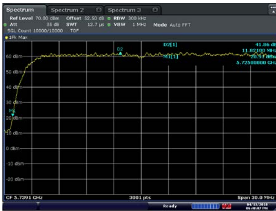
Figure 8.2-7: - Lower band edge emissions at 5725 MHz, 30 MHz Channel BW, Low channel (Marker-delta method)
