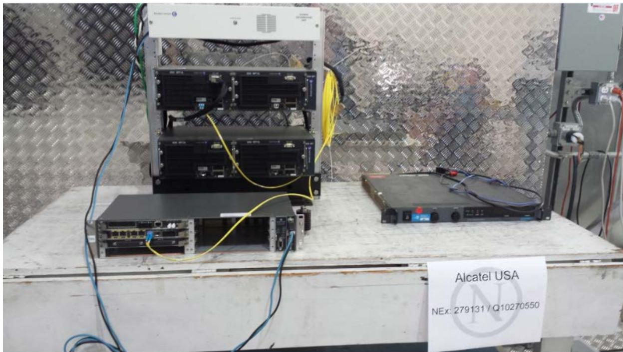
**Rear of Powerline Conducted Emissions Setup**
