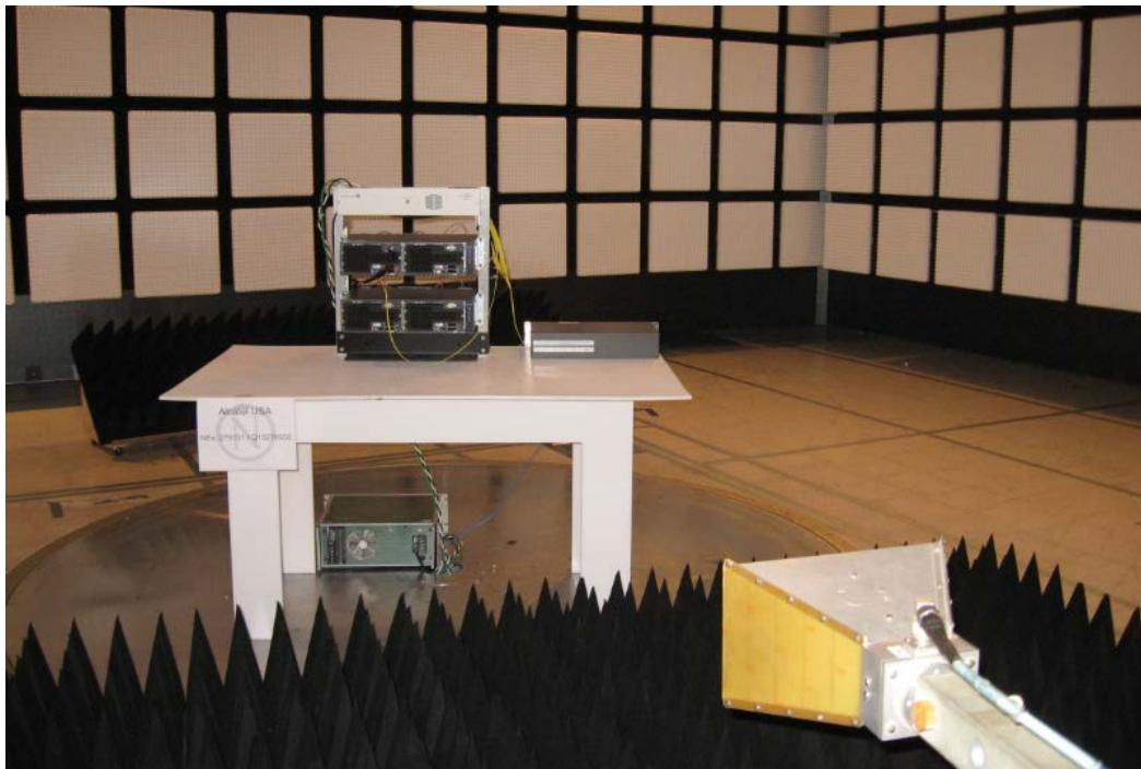
**Rear of Radiated Emissions Setup**
