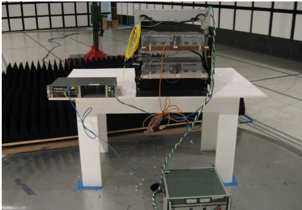
**Front of Powerline Conducted Emissions Setup**
