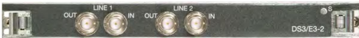
Figure 6-82. P2E3DS3 PDH card front panel
