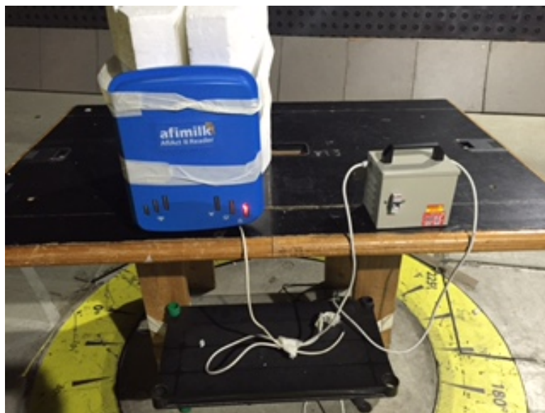
Photograph 8.2.2 Setup for radiated emission measurements, EUT cabling
