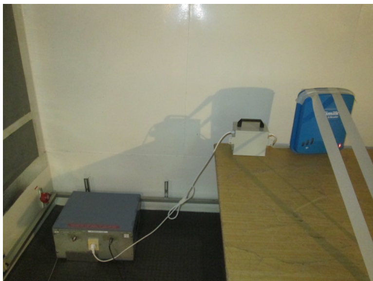
Photograph 8.1.1 Setup for conducted emission measurements
