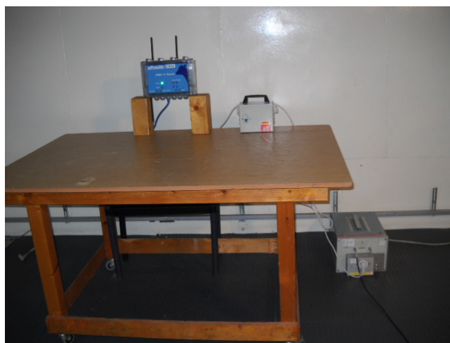
Photograph 8.1.1 Setup for conducted emission measurements
