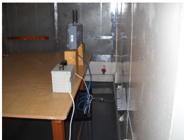
Photograph 8.1.1 Setup for conducted emission measurements
