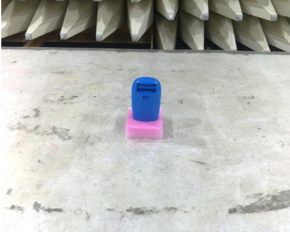
Photograph No.4 Setup for spurious emission field strength measurements, EUT close view
