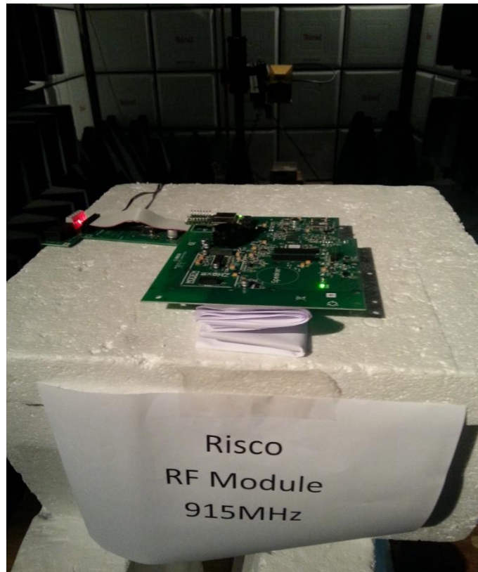
Figure 6. Radiated Emission Test
