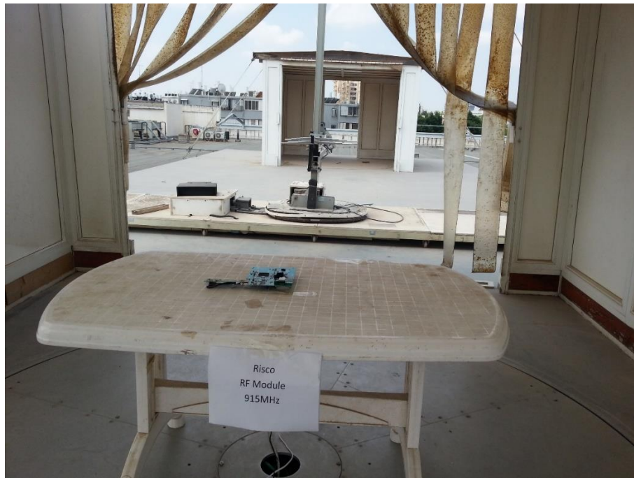
Figure 4. Radiated Emission Test
