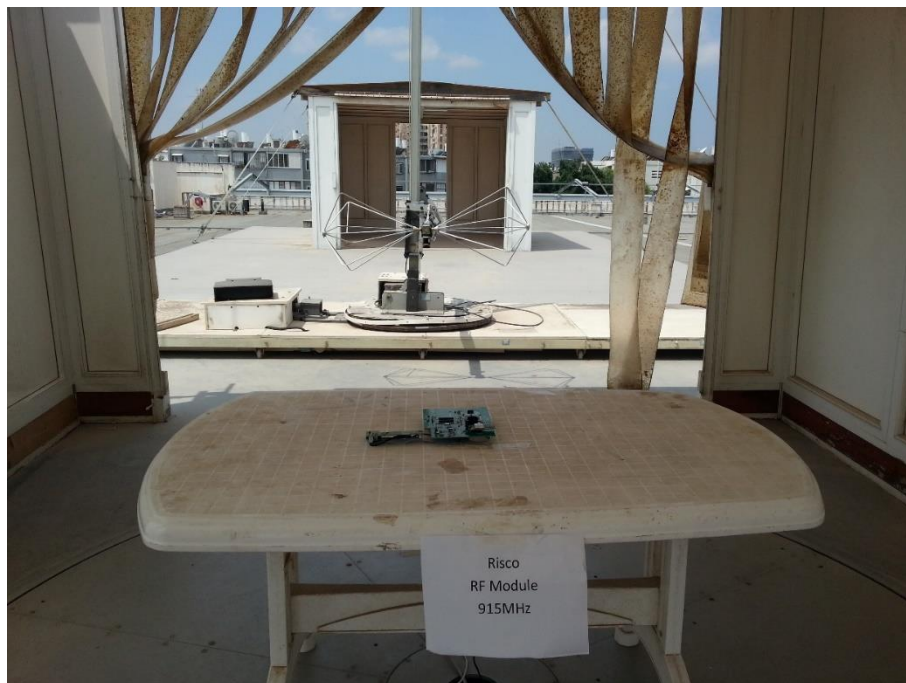
Figure 5. Radiated Emission Test
