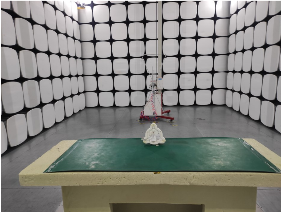
Radiated Emission test view (Frequency from 1GHz to 18GHz)
