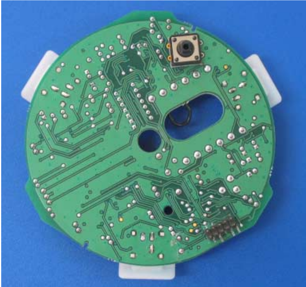
Photograph No.5 RK200DT0000A detector, print side of the main PCB
