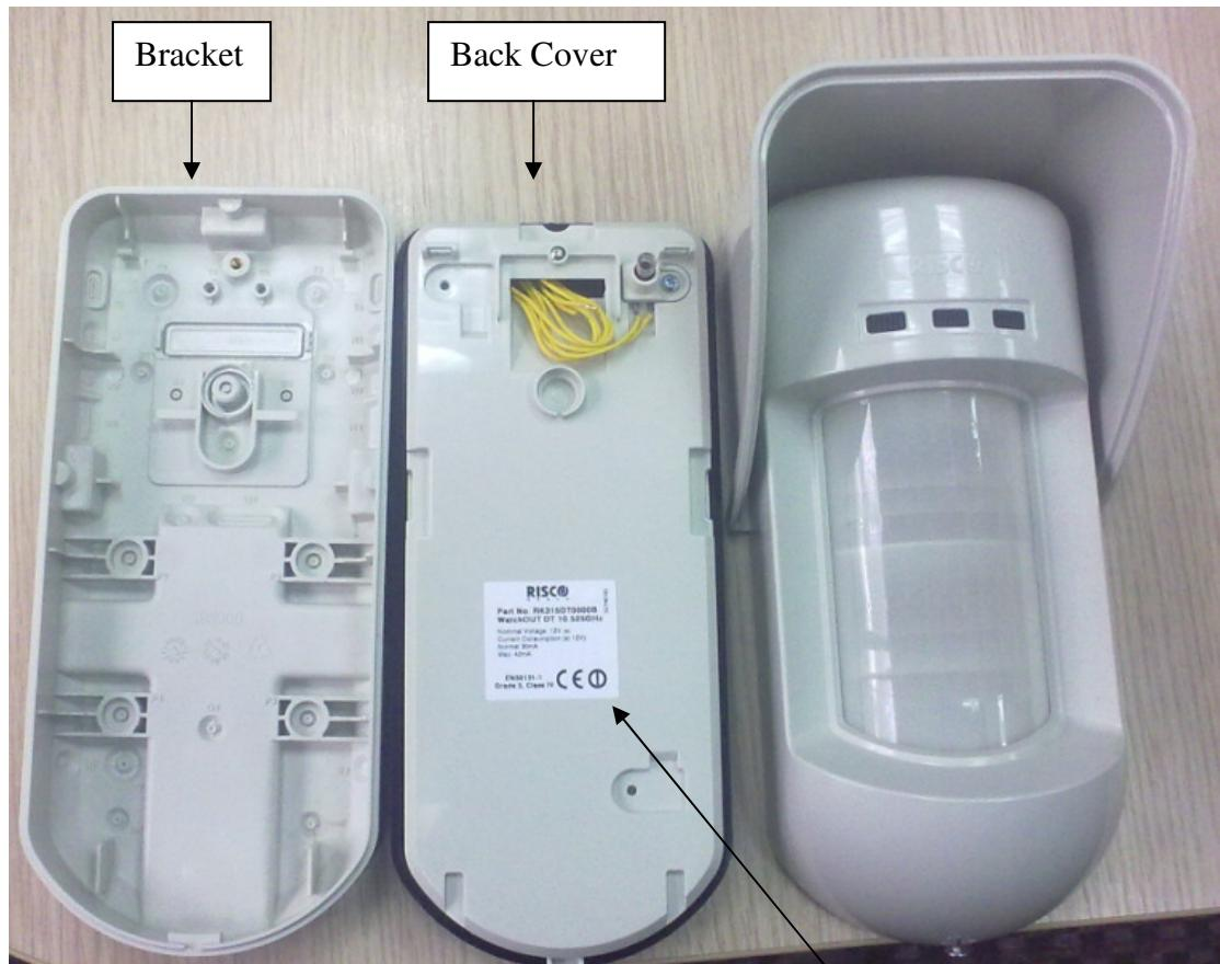
The back cover is located inside the bracket.
