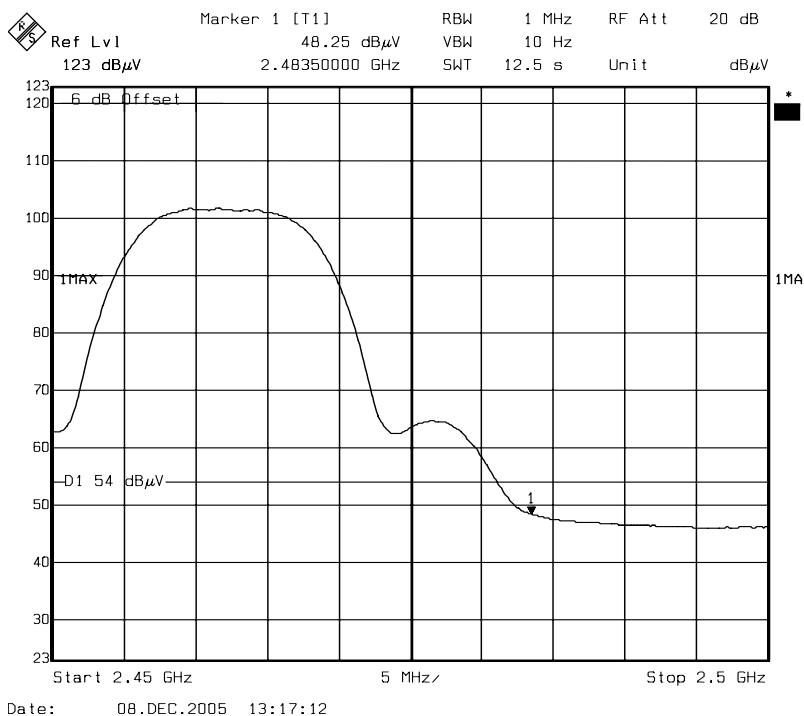
**Band Edges (IEEE 802.11g mode / CH Low)****Detector mode: Peak    Polarity: Vertical**
