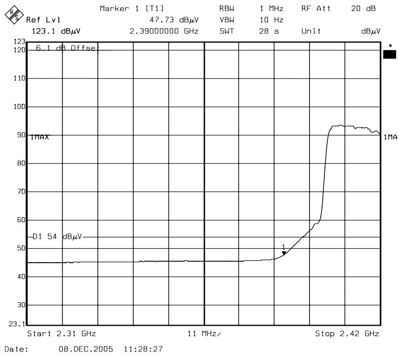
**Band Edges (IEEE 802.11g mode / CH High)****Detector mode: Peak    Polarity: Vertical**
