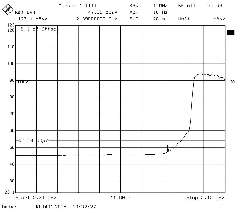
**Detector mode: Peak    Polarity: Horizontal**
