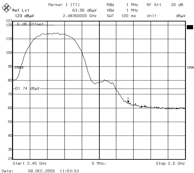
**Detector mode: Average    Polarity: Vertical**
