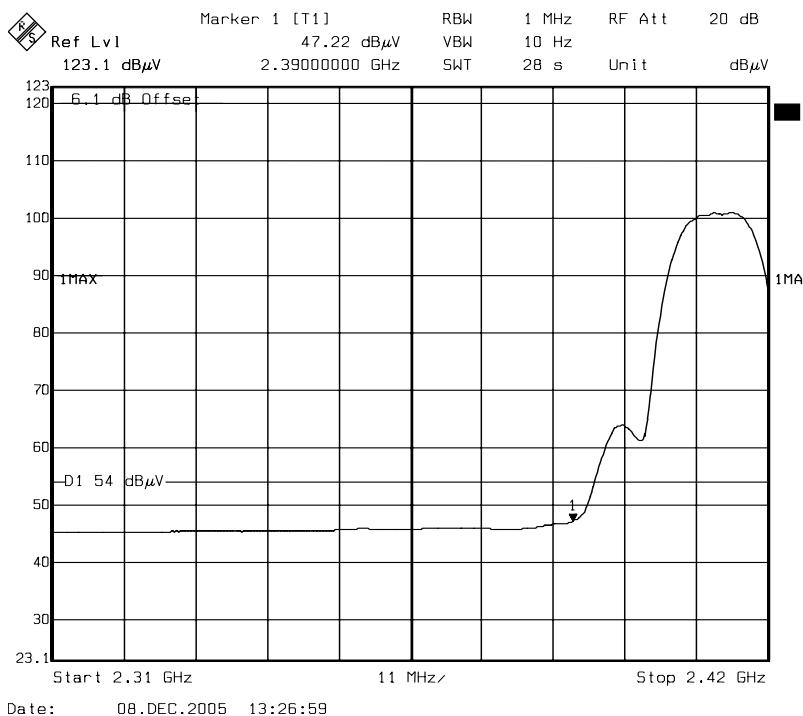
**Band Edges (IEEE 802.11b mode / CH High)****Detector mode: Peak    Polarity: Vertical**
