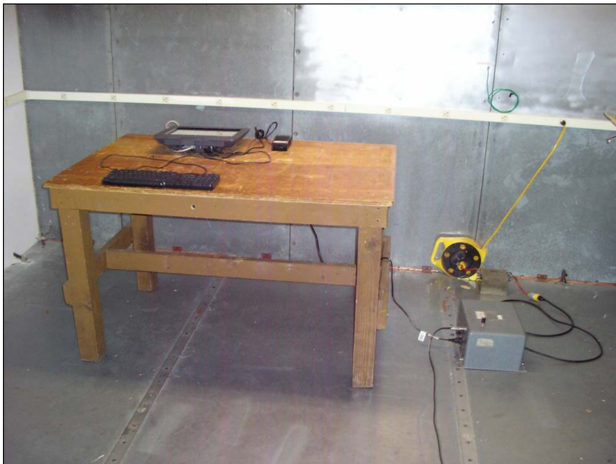
Photograph 2. Conducted Emissions, 15" Model, Test Setup
