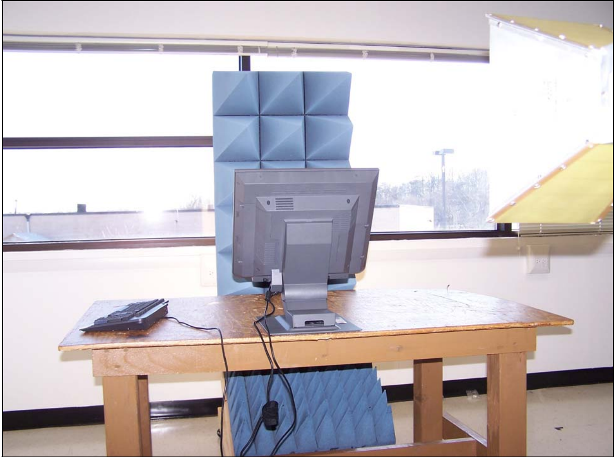
Photograph 5. Radiated Emissions, 15" Model, Test Setup
