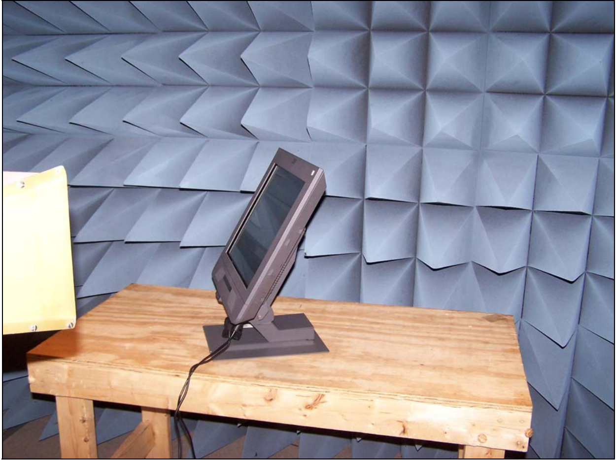
Photograph 6. Radiated Emissions, 17" Model, Test Setup
