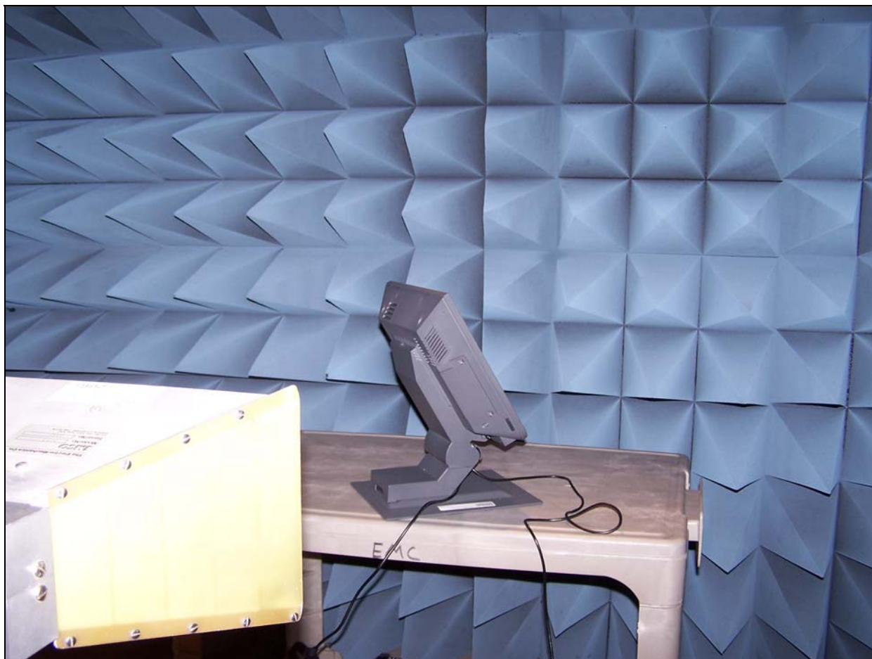
Photograph 4. Radiated Emissions, 12" Model, Test Setup
