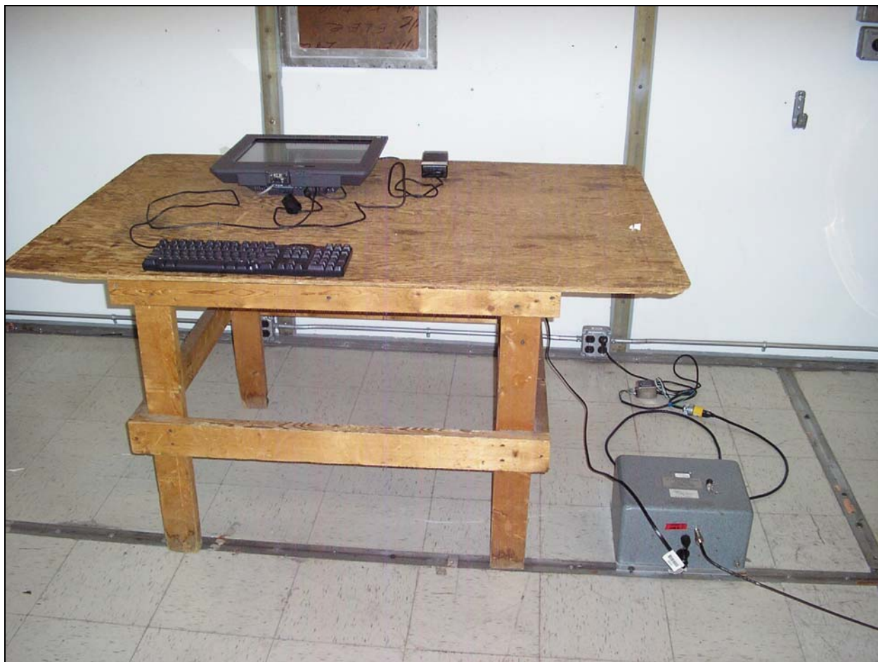
Photograph 3. Conducted Emissions, 17" Model, Test Setup
