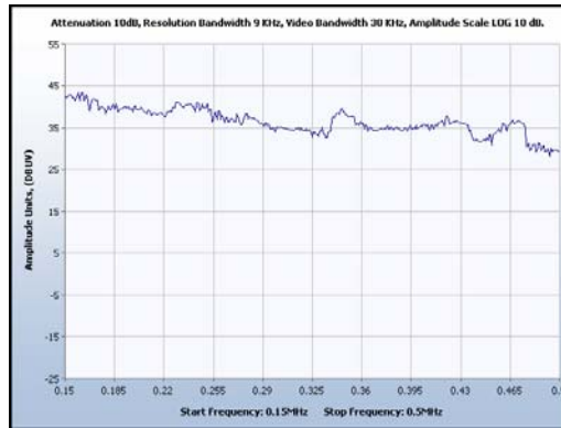
Plot 41. Conducted Emissions - Voltage, 12" Model, Phase Line Plot (120VAC, 60Hz), Channel 6, 802.11 g, 0.15 MHz – 0.5 MHz
