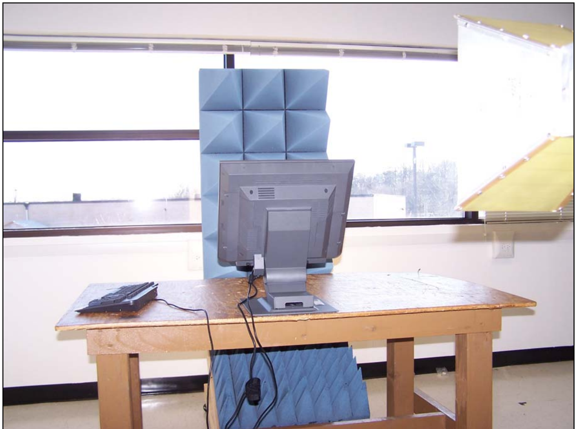
Photograph 9. Radiated Emissions, 15" Model, Test Setup
