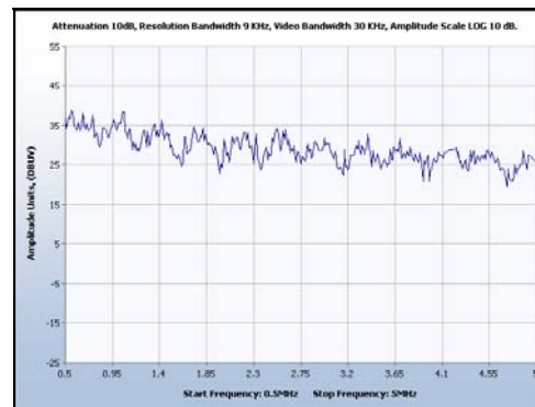
Plot 81. Conducted Emissions - Voltage, 17" Model, Neutral Line Plot (120VAC, 60Hz), Channel 6, 802.11 g, 0.5 MHz – 5 MHz
