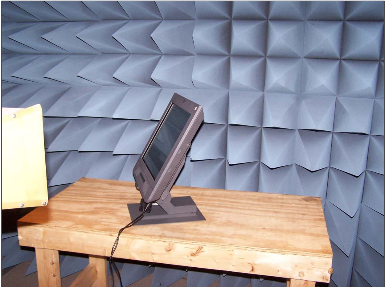
Photograph 10. Radiated Emissions, 17" Model, Test Setup
