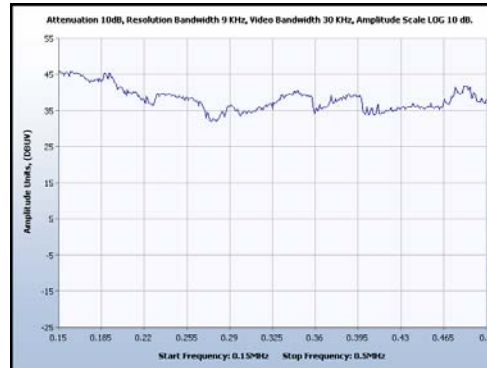
Plot 80. Conducted Emissions - Voltage, 17" Model, Neutral Line Plot (120VAC, 60Hz), Channel 6, 802.11 g, 0.15 MHz – 0.5 MHz
