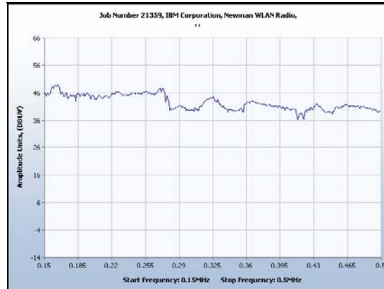
Plot 86. Conducted Emissions - Voltage, 17" Model, Neutral Line Plot (120VAC, 60Hz), Channel 11, 802.11g, 0.15 MHz – 0.5 MHz
