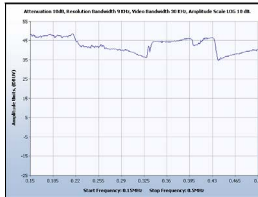
Plot 68. Conducted Emissions - Voltage, 15" Model, Neutral Line Plot (120VAC, 60Hz), Channel 11, 802.11g, 0.15 MHz – 0.5 MHz
