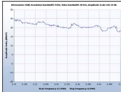
Plot 35. Conducted Emissions - Voltage, 12" Model, Phase Line Plot (120VAC, 60Hz), Channel 1, 802.11 g, 0.15 MHz – 0.5 MHz
