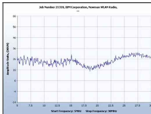
Plot 88. Conducted Emissions - Voltage, 17" Model, Neutral Line Plot (120VAC, 60Hz), Channel 11, 802.11 g, 5 MHz – 30 MHz
