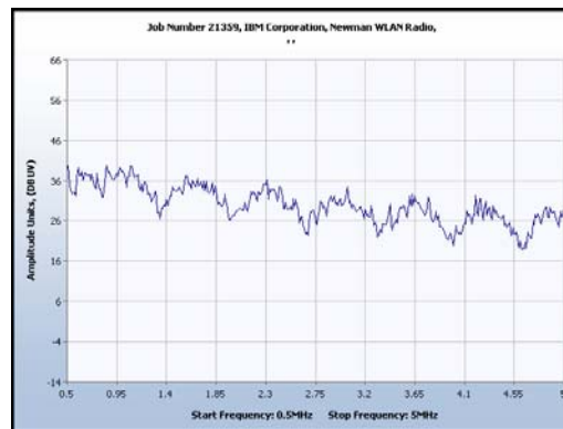
Plot 87. Conducted Emissions - Voltage, 17" Model, Neutral Line Plot (120VAC, 60Hz), Channel 11, 802.11 g, 0.5 MHz – 5 MHz
