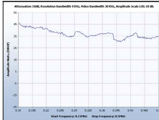
Plot 53. Conducted Emissions - Voltage, 15" Model, Phase Line Plot (120VAC, 60Hz), Channel 1, 802.11 g, 0.15 MHz – 0.5 MHz
