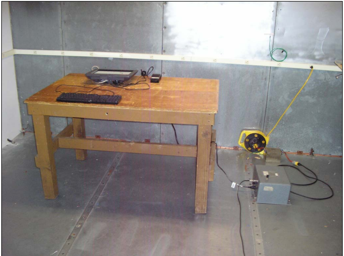
Photograph 6. Conducted Emissions, 15" Model, Test Setup
