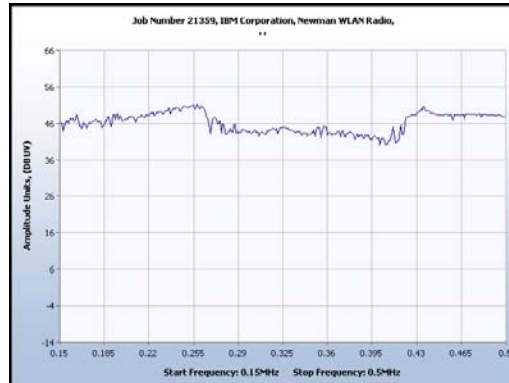
Plot 83. Conducted Emissions - Voltage, 17" Model, Phase Line Plot (120VAC, 60Hz), Channel 11, 802.11 g, 0.15 MHz – 0.5 MHz
