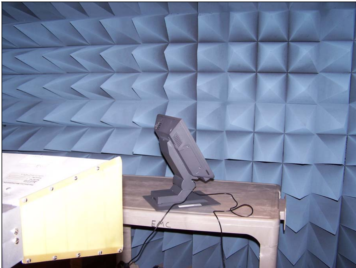
Photograph 8. Radiated Emissions, 12" Model, Test Setup
