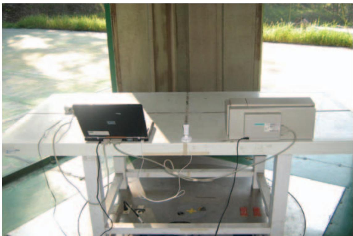
**RADIATED RF MEASUREMENT SETUP**
