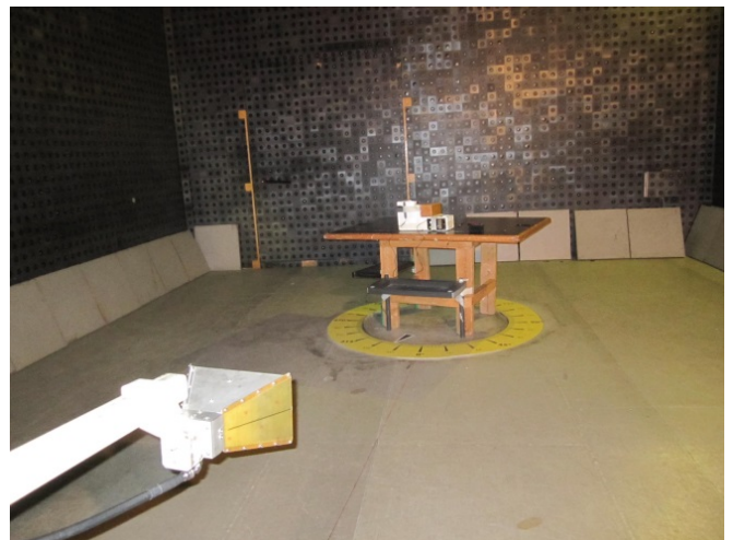
Photograph 8.1.1 Setup for preliminary radiated emission measurements
