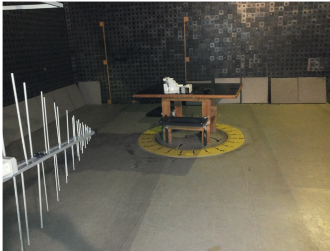
Photograph 8.1.1 Setup for preliminary radiated emission measurements
