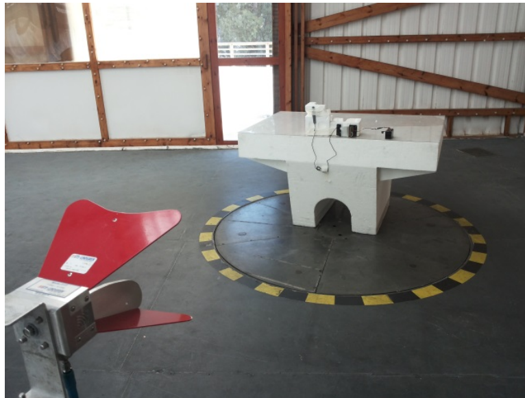
Photograph 8.1.2 Setup for final radiated emission measurements, general view
