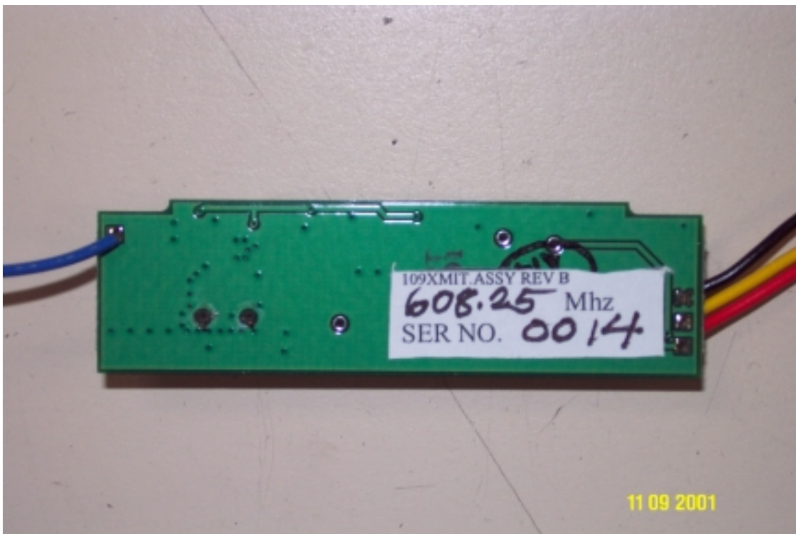
Rear view: Transmitter board.
