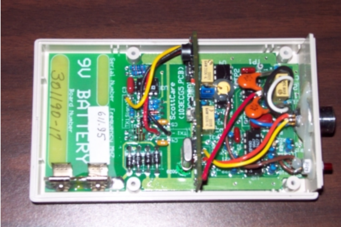
Internal view: Inside view of the transmitter board and the ECG5 (ScottCare) board. The combination of the two boards transmits data to the receiver.
