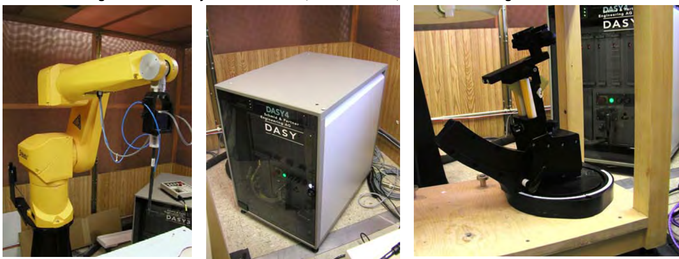
Figure 5-1 DASY4 system: Robot Arm, Controller box, Device Positioning Holder
