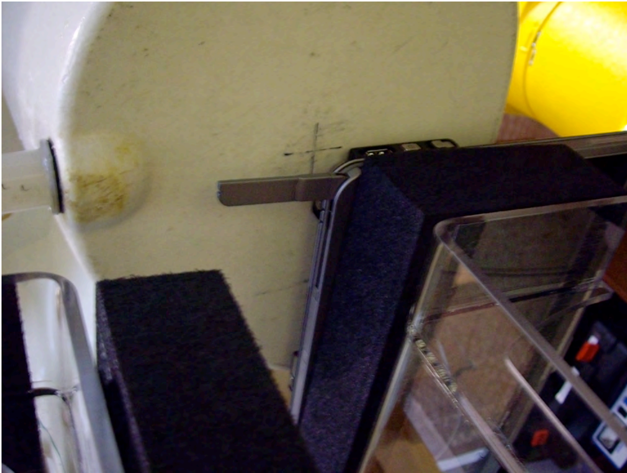
Figure 12-8 Notebook positioned under Phantom, antenna in 90° position
