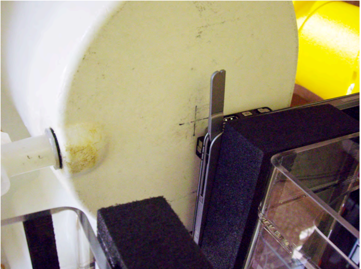
Figure 12-9 Notebook positioned under Phantom, antenna in 180° position
