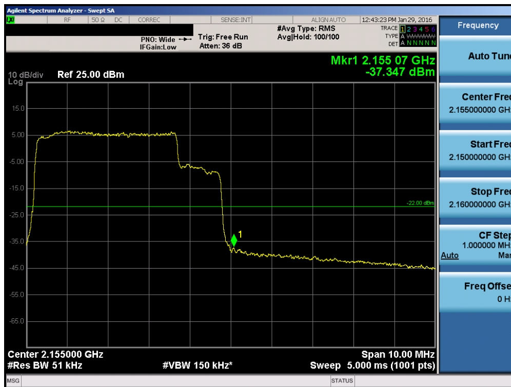
Plot 7-60. Upper Band Edge Plot (Band 4 – 5.0MHz QPSK – RB Size 25)
