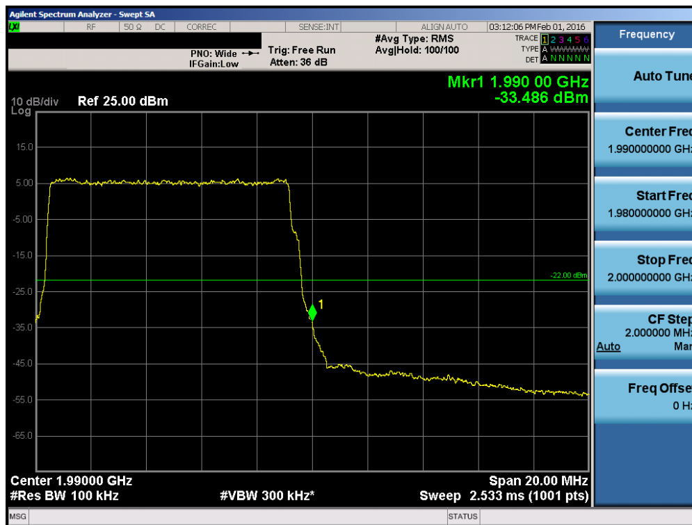
Plot 7-80. Upper Band Edge Plot (Band 2 – 10.0MHz QPSK – RB Size 50)
