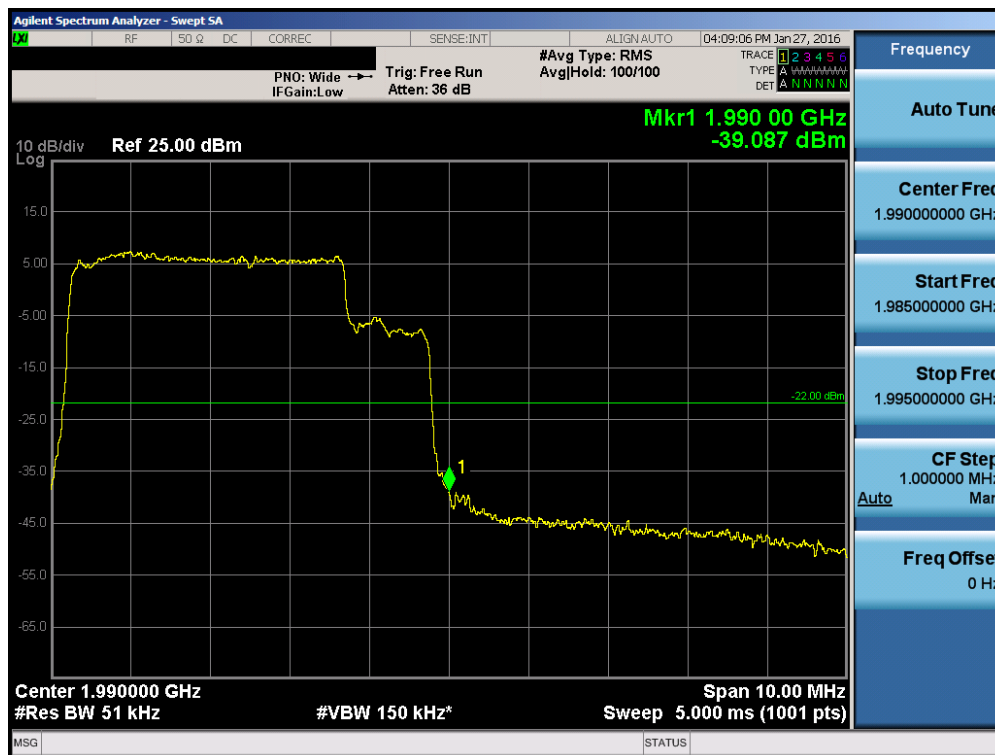
Plot 7-44. Upper Band Edge Plot (Band 2 – 5.0MHz QPSK – RB Size 25)
