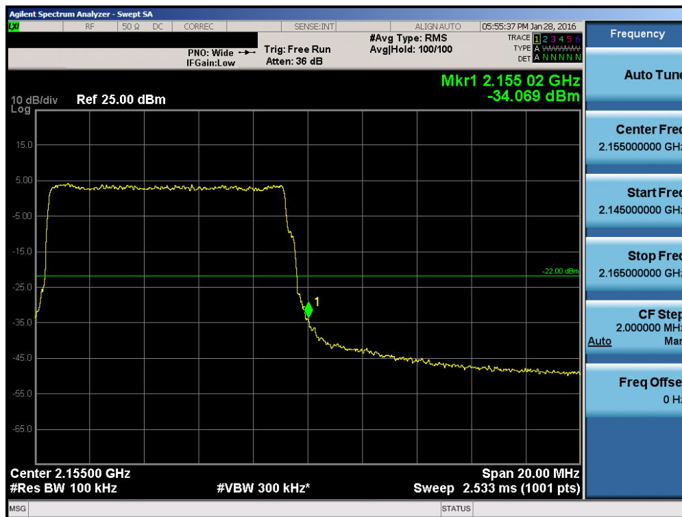
Plot 7-32. Upper Band Edge Plot (Band 4 – 10.0MHz QPSK – RB Size 50)
