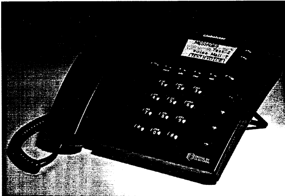
Figure 2-4 Typical Fixed Terminal Desk Set
