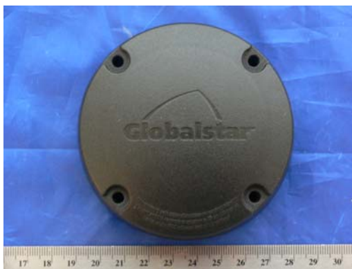
Passive TX/RX Patch Antenna View
