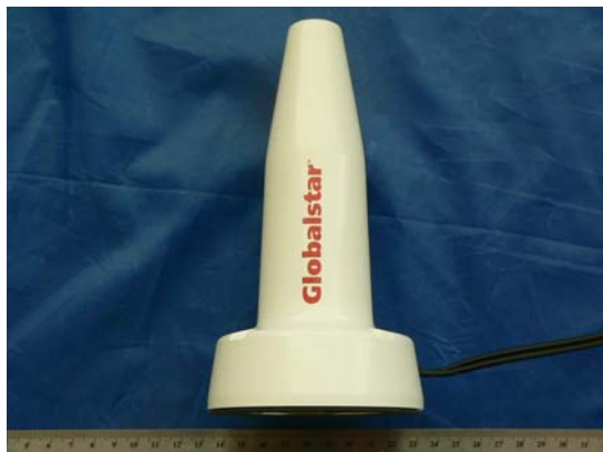
Active TX/RX Quadrafilament Helix (QFH) View
