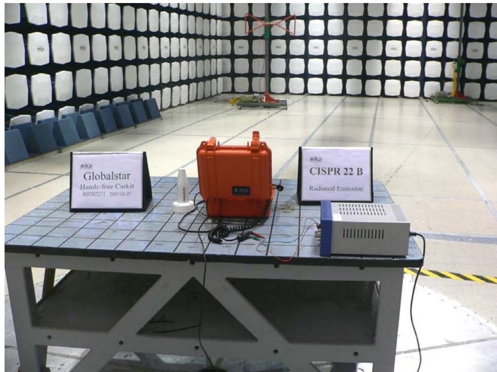
**Transmitter Radiated Emission- Front View**
