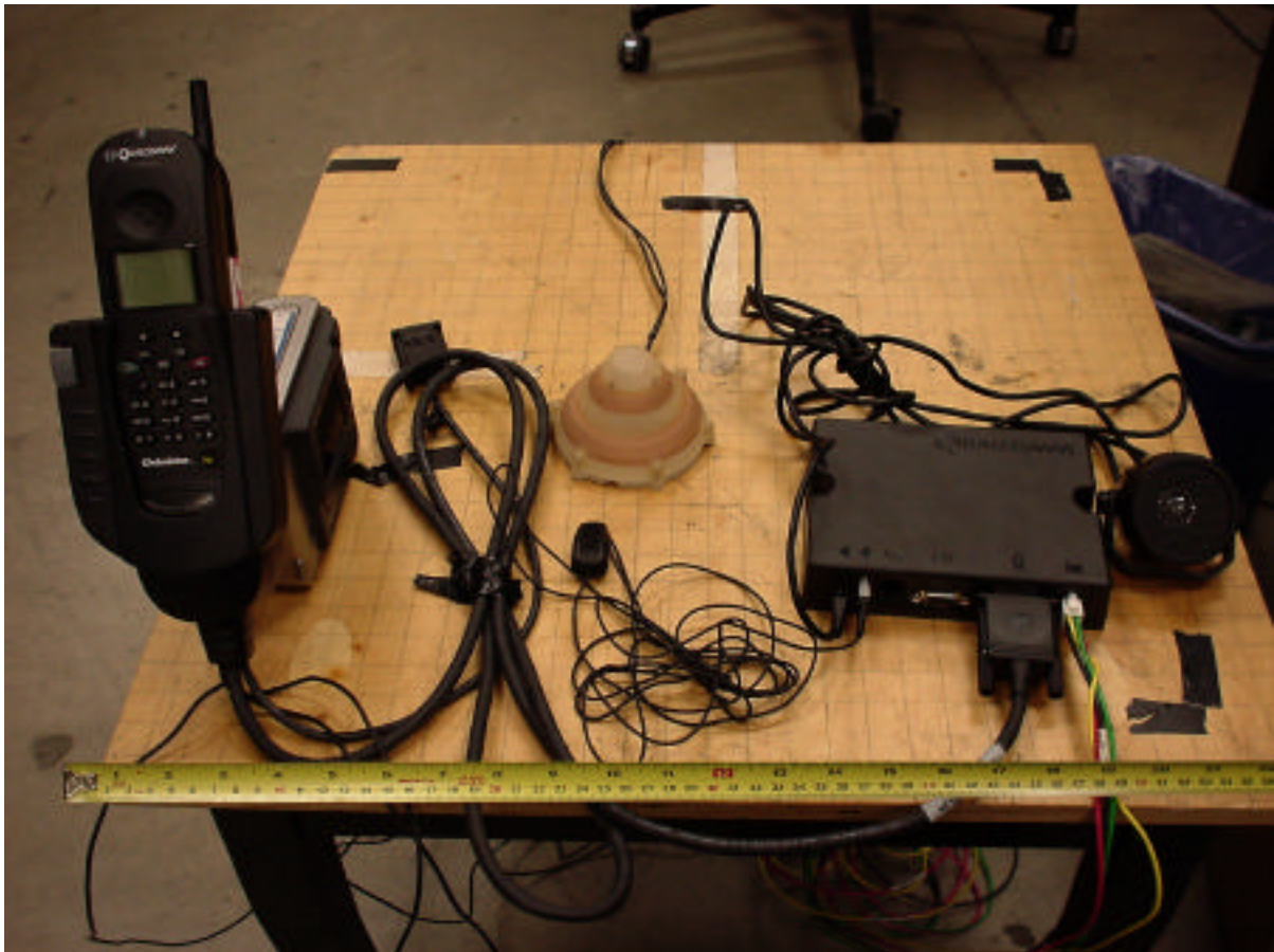
Photo C-1 GCK 1410 Car Kit Components
