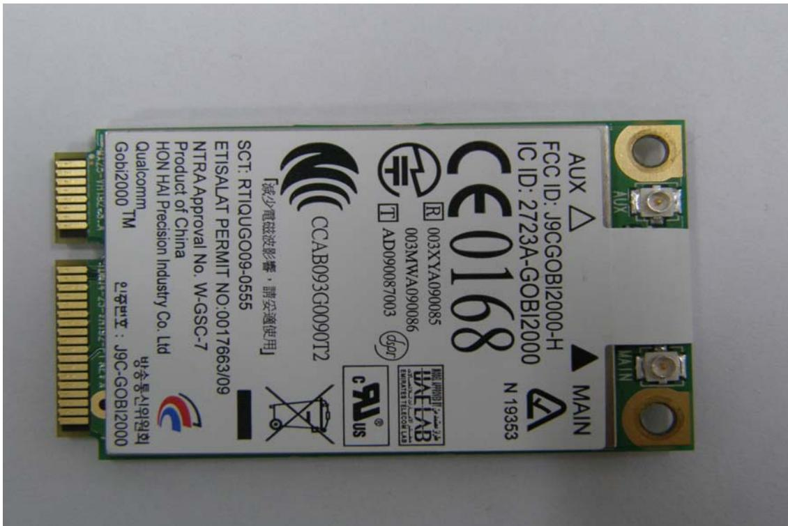
*Internal View of EUT-3 (WWAN Module)*
