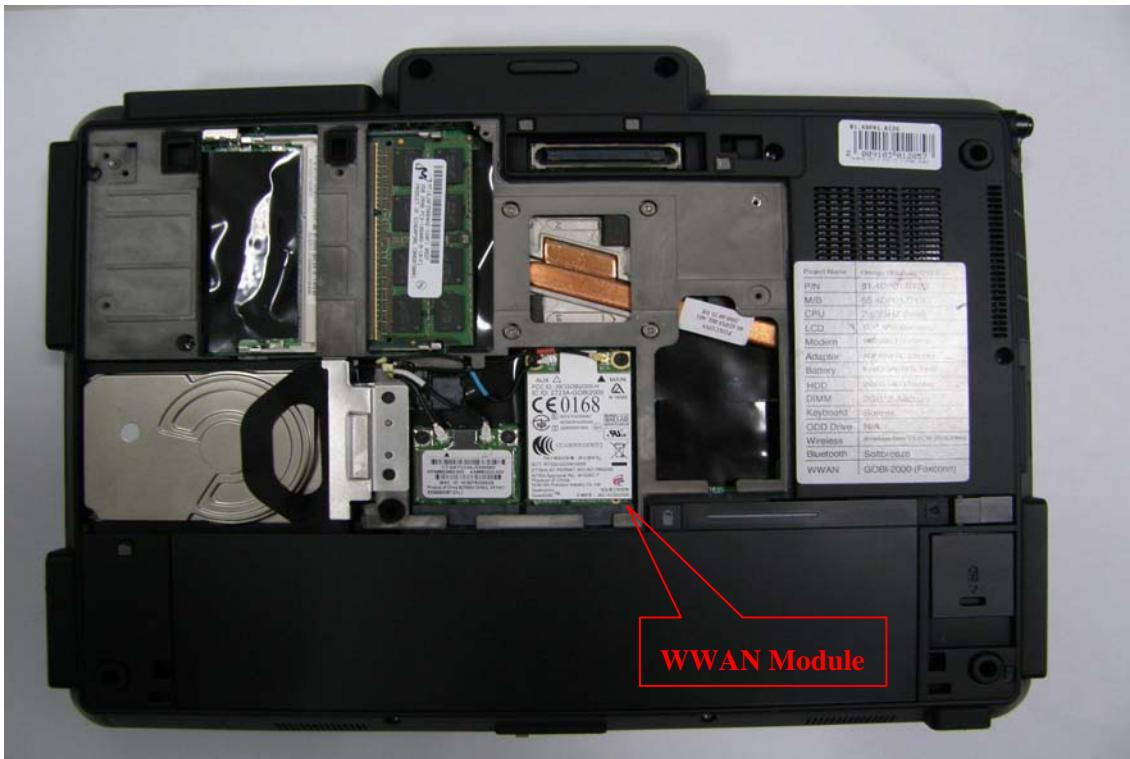
*Internal View of EUT -1 (WWAN Module)*
