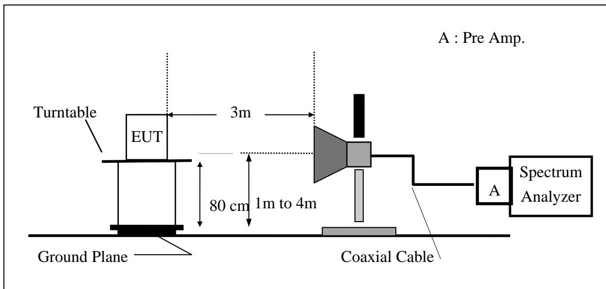
(C) Substituted Method Test Set-UP
