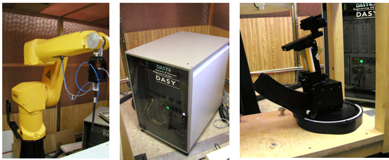
Figure 5-1 DASY4 system: Robot Arm, Controller box, Device Positioning Holder
