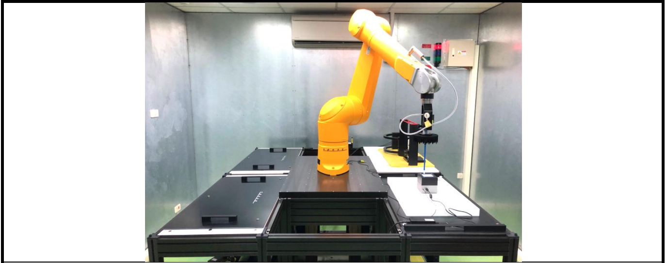
Fig-3.2 SPEAG DASY6 System
