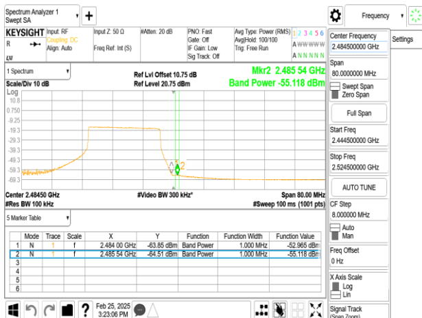
SISO 802.11ax 40MHz Chain0 2462MHz RU484
