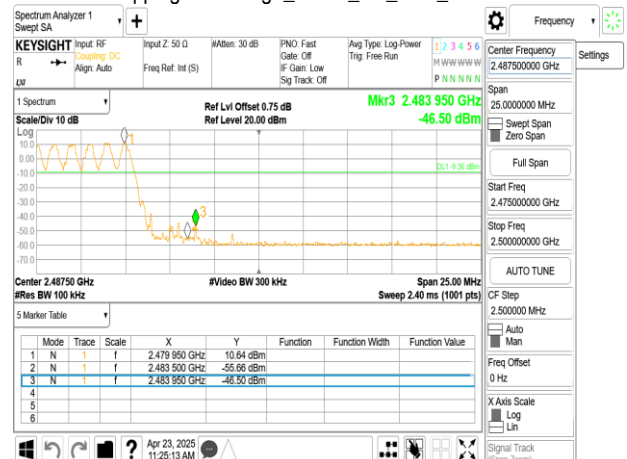
Hopping Band Edge_GFSK_1M_DH5_2480MHz
