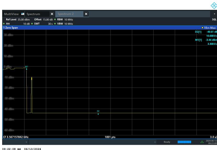
**[Step 5] Configure SAS granted CBSD to operate at frequency 3650-3690 MHz & power level 20 dBm/MHz**
