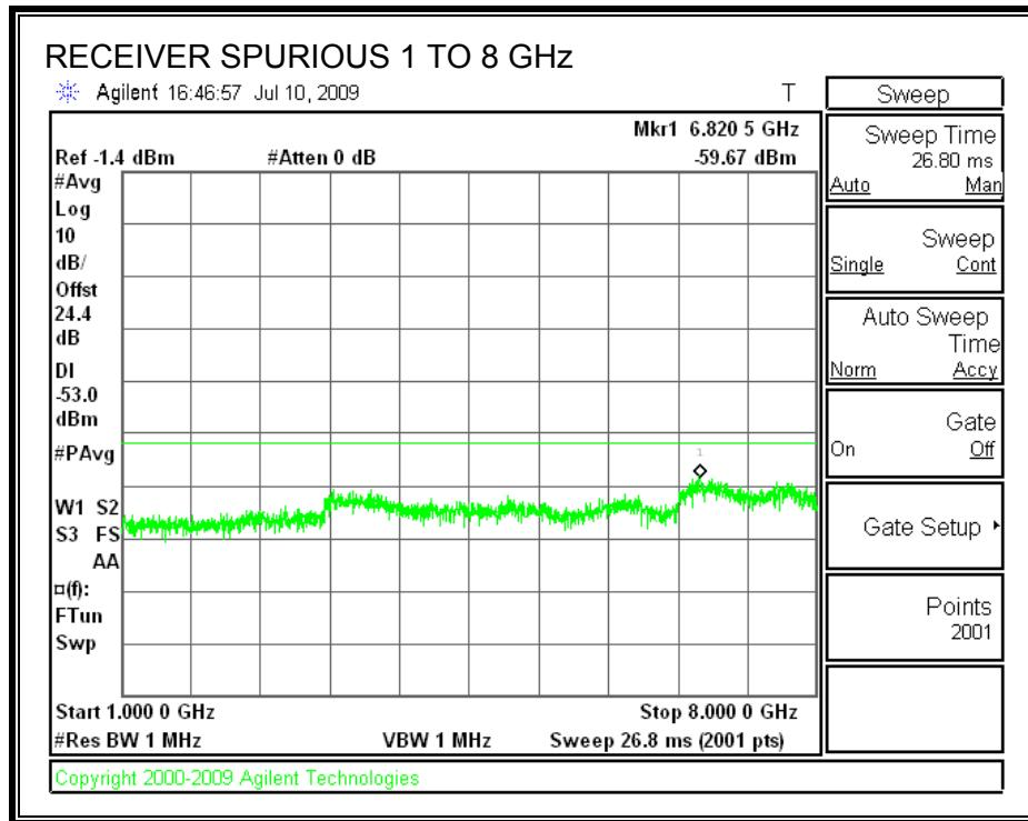
**RECEIVER SPURIOUS EMISSIONS IN THE 5.8 GHz BAND**
