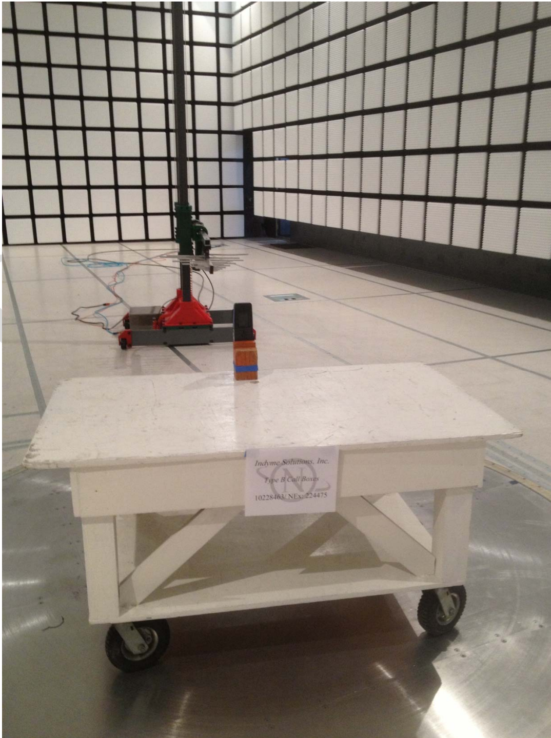
Radiated Field Strength Spurious Emission Test Setup
