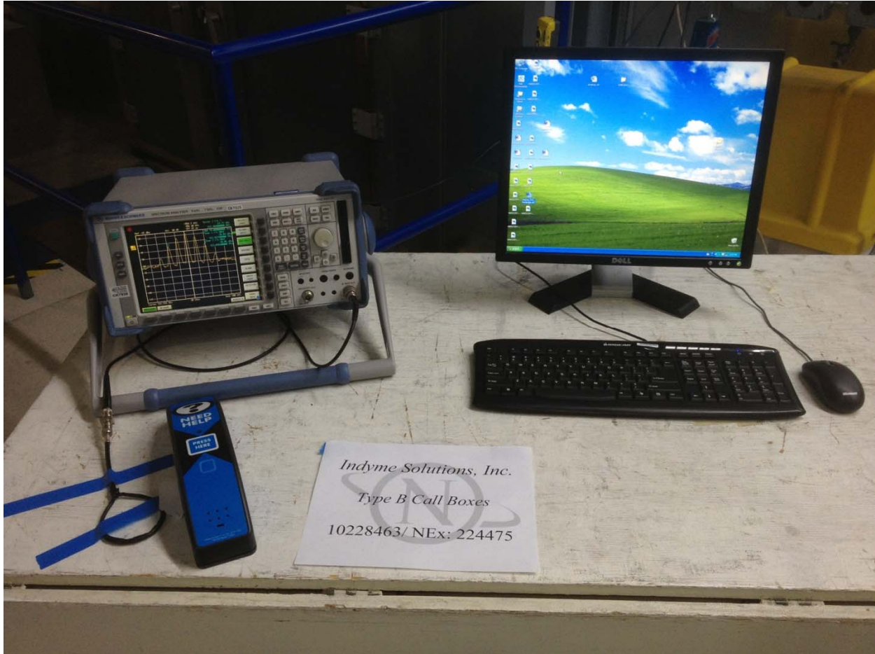
Occupied Bandwidth Test Setup
