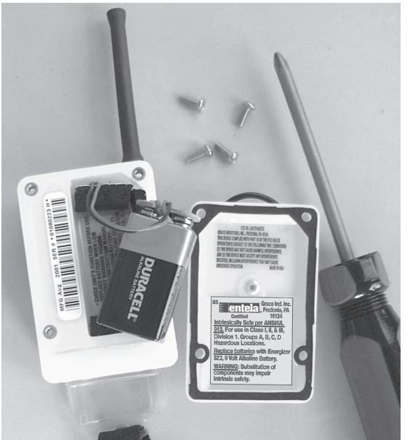
To reduce the risk of ignition of a flammable atmosphere, batteries must only be changed in an area known to be non-flammable. To change the battery, remove the four screws securing the back. Remove the back cover, disconnect and dispose of the spent battery and connect the new battery. Replace the back cover and gently tighten all four screws using a criss-cross pattern for even gasket pressure ensuring a good seal. Do not over tighten screws.
