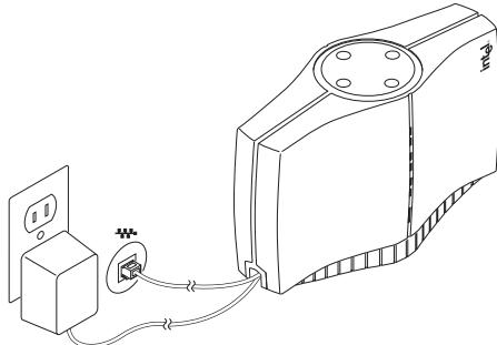
Set the access point on a flat surface such as a table or desk. If the access point is positioned on a desk or table, the antenna should be on top (as shown above).
