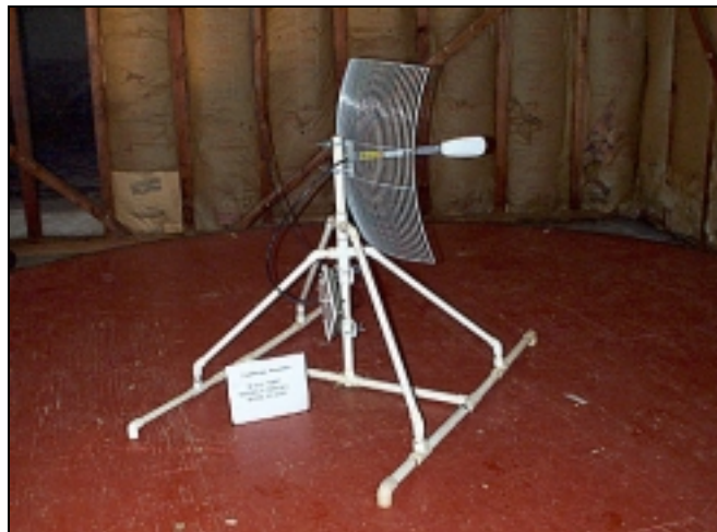
Transmitter with Parabolic Antenna
