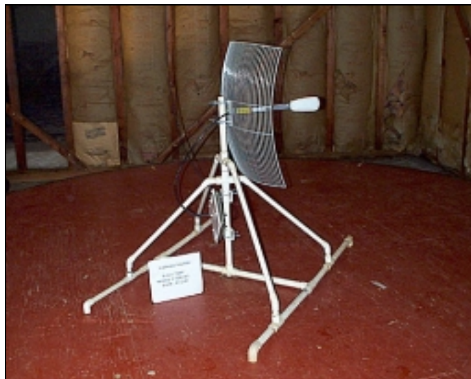
Transmitter with Parabolic Antenna
