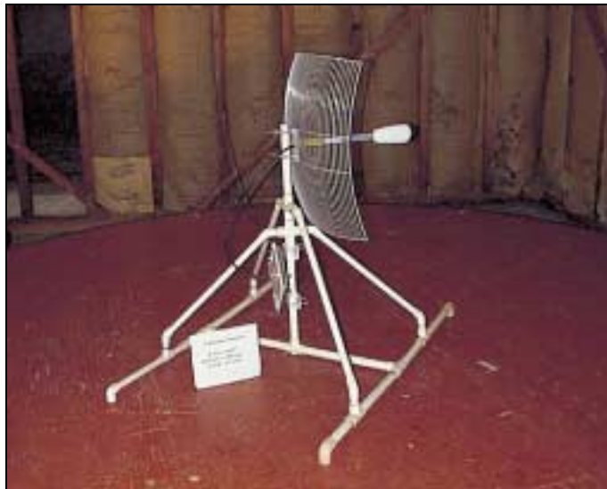
Transmitter with Parabolic Antenna
