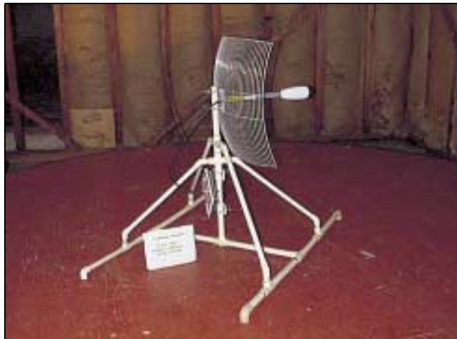
Transmitter with Parabolic Antenna
