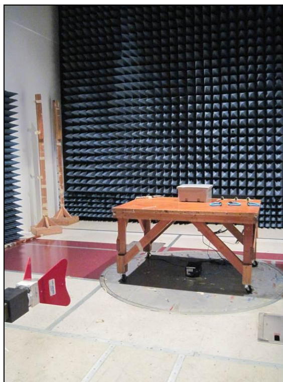
Photograph 3. Radiated Emission, Test Setup, 1 GHz – 10 GHz
