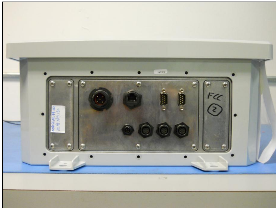
Photograph 2. Echelon Corporation Edge Control Node (ECN) 70101-0026, Rear View
