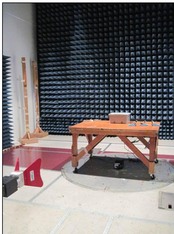
Photograph 3. Radiated Emission, Test Setup, 1 GHz – 10 GHz
