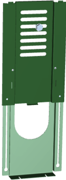
Figure 6. Attach the Mounting Bracket to the Transformer's Lifting Nut
