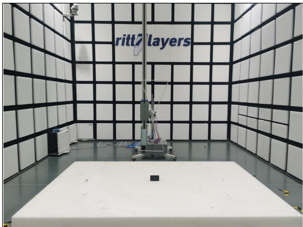
Radiated emission test: Frequency Range< Above 960MHz >
