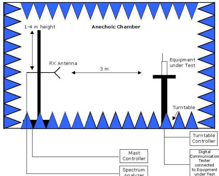
Drawing 1: Setup in the Anechoic chamber. For measurements below 1 GHz the ground was replaced by a conducting ground plane.
