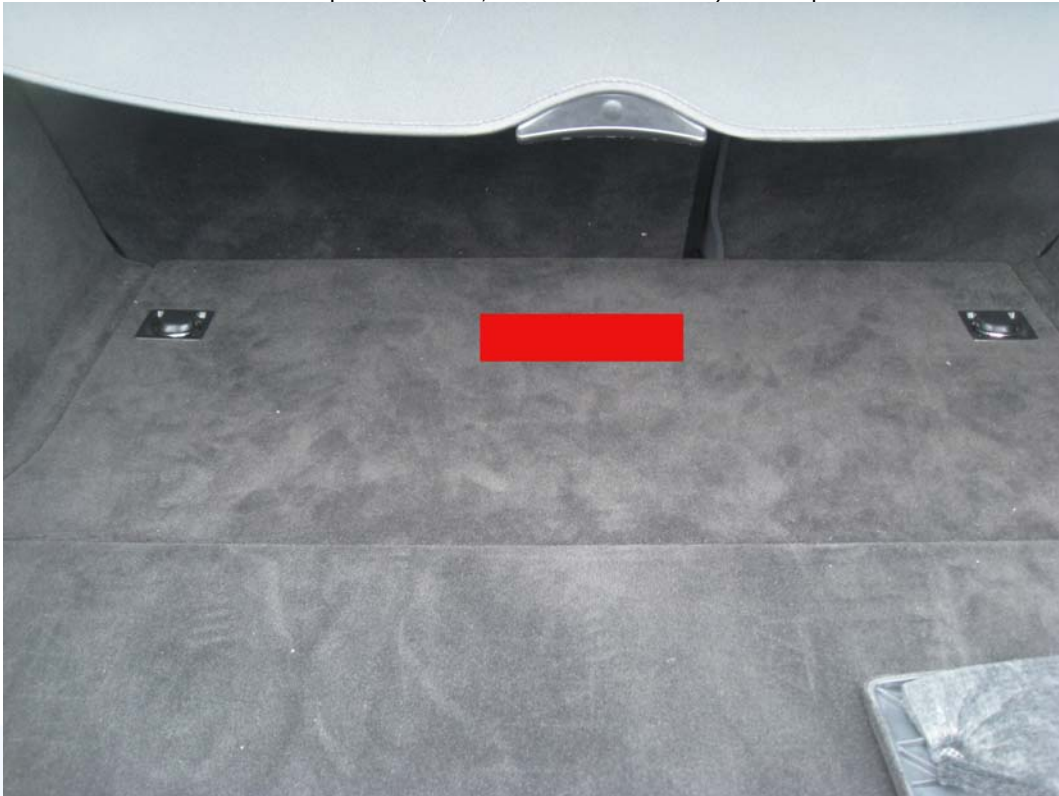
LF antenna position (trunk; behind the back seat) – red square
