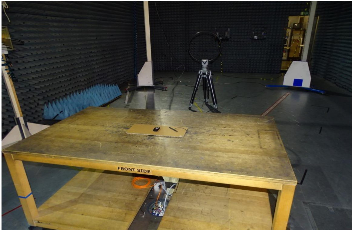
Photo 1: Test setup for radiated measurements below 30 MHz
