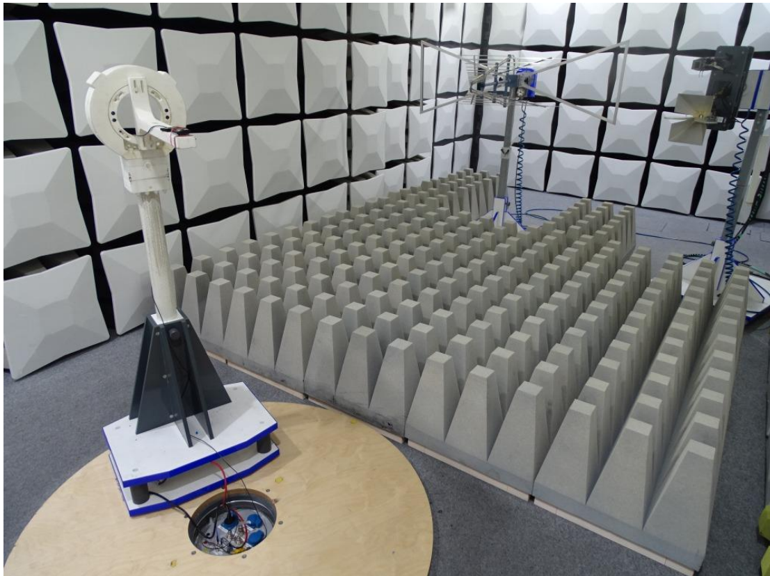
Photo 3: Test setup for radiated measurements above 1 GHz
