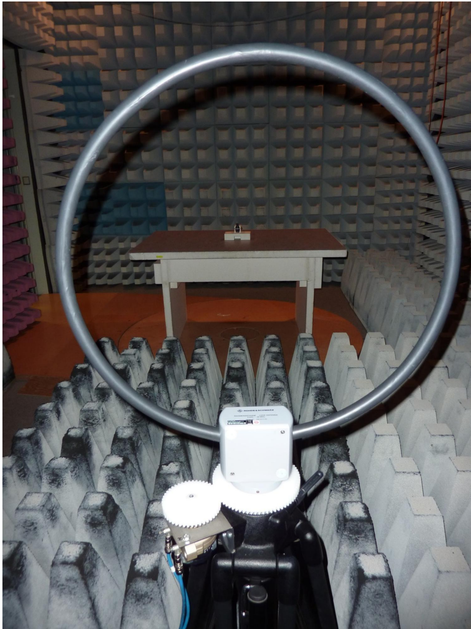
153783_1.JPG: Test setup fully anechoic chamber
