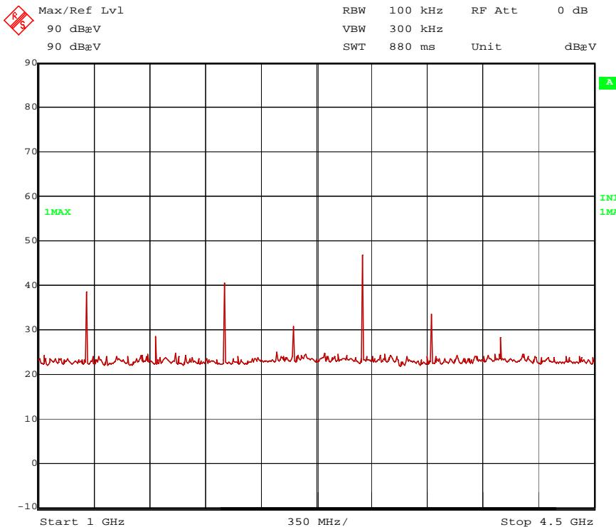
The following frequencies were found during the preliminary radiated emission test:
