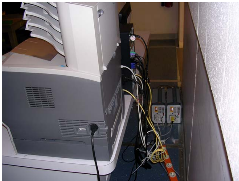
Figure 59. Test configuration for transmitter conducted emissions (side view).
