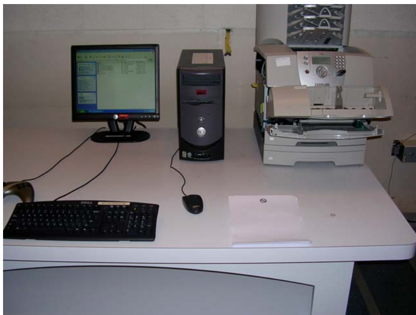
Figure 58. Test configuration for transmitter conducted emissions (front view).
