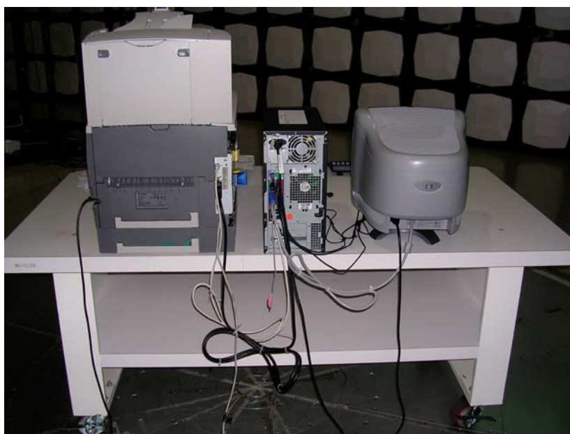
Figure 57. Test configuration for transmitter spurious emissions (back view).
