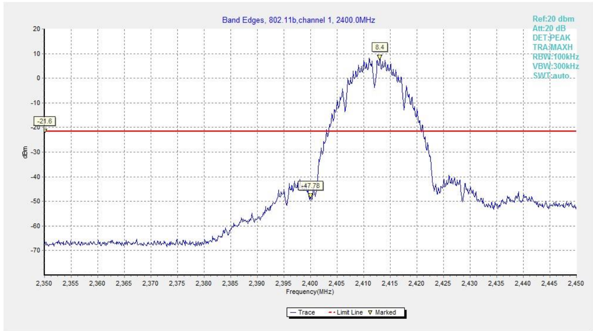
Fig.19 Band Edges (802.11b, CH 1)
