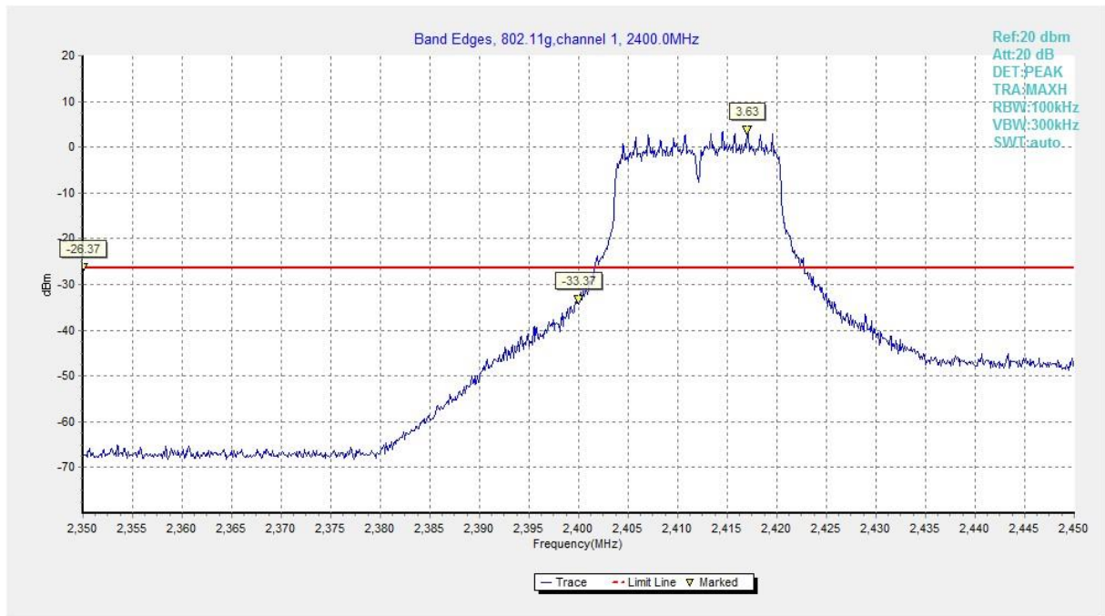
Fig.21 Band Edges (802.11g, CH 1)
