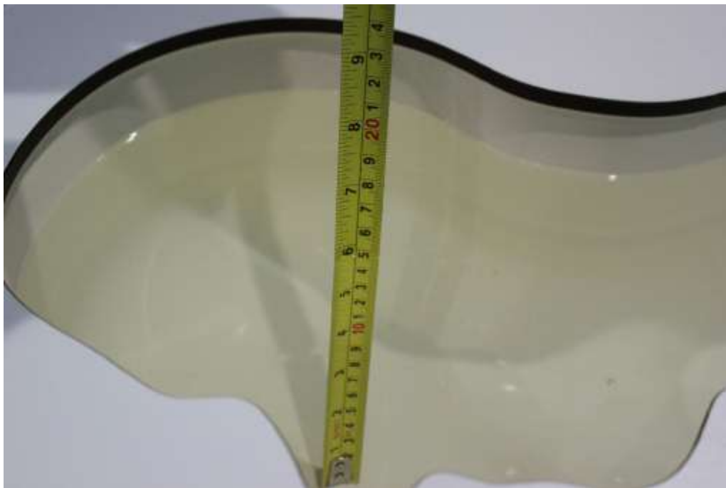
Picture 7-2: Liquid depth in the Head Phantom(5GHz)
