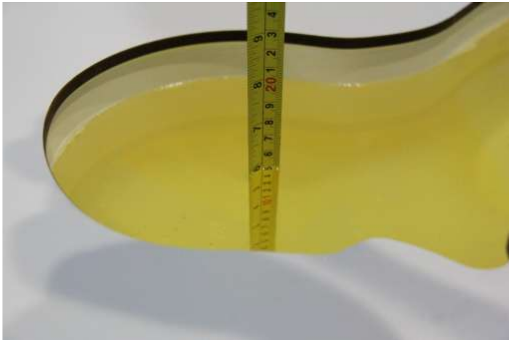
Picture 7-1: Liquid depth in the Head Phantom(2450MHz)
