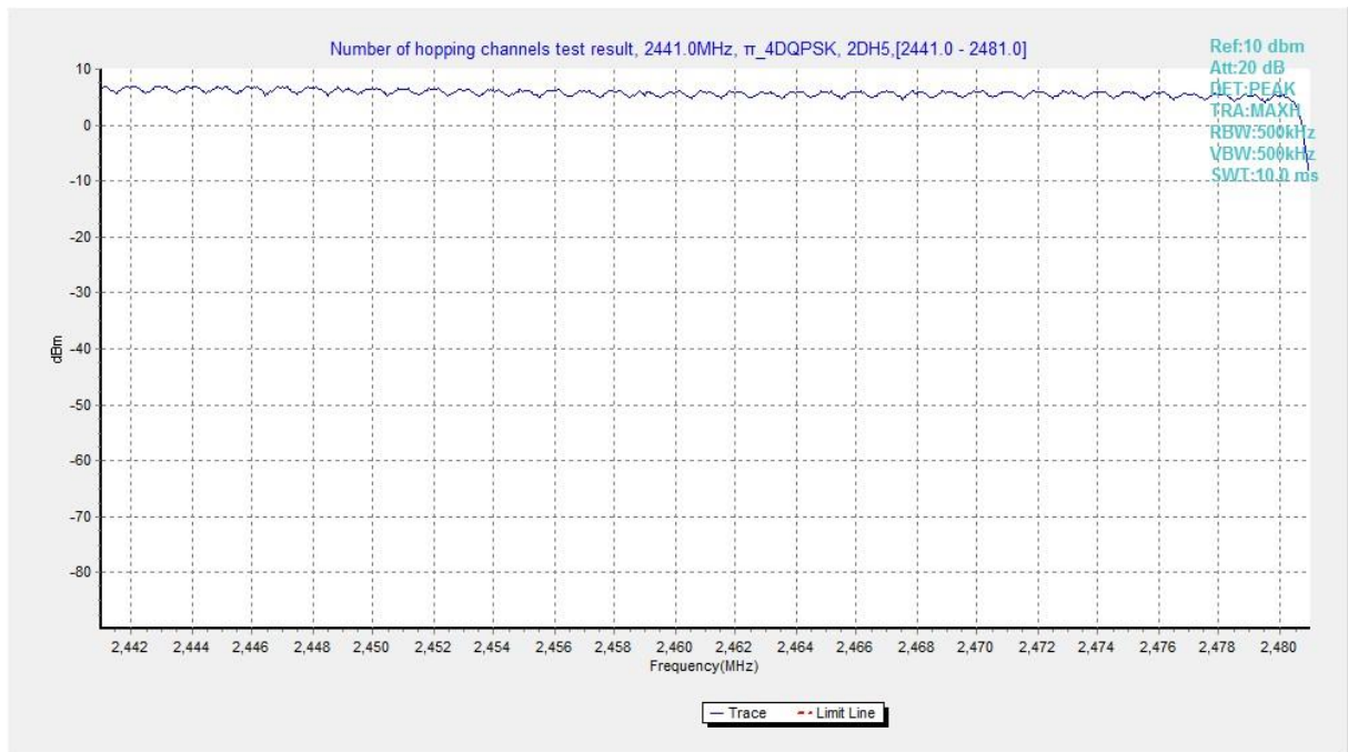
Fig. 78 Hopping channel ch39~78 ( \pi/4 DQPSK, Ch39)
